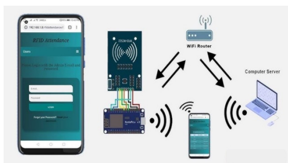
Gambar 2. Smart Attendance System berbasis RFID dan Face Recognition
